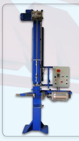
The SVA C02 helps with the tightening and unscrewing of valves on any C02 tank. It has a pneumatic vise that can block 2-50 Kg tanks. The locking is automatic and can be setted with a keyboard. Controls are bimanual, in compliance with safety standards.
