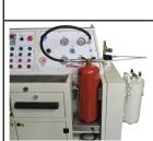
Hydraulic cylinder test: maintain hydraulic pressure at "PT" for 30 seconds and proceed with depressurization.
