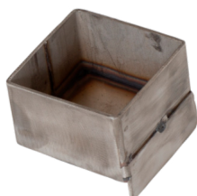
STAINLESS STEEL CONTAINER FOR FIRE SIMULATOR IGNITION
